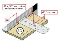
E. Windows using frame screws: Pre-drill installation screw holes. On the room side of the window, drill 13/64" diameter clearance holes through the frame as shown on the placement diagram. Space the holes a maximum of 6" from each end and a maximum of 10" on center on the head, jambs and sill.
